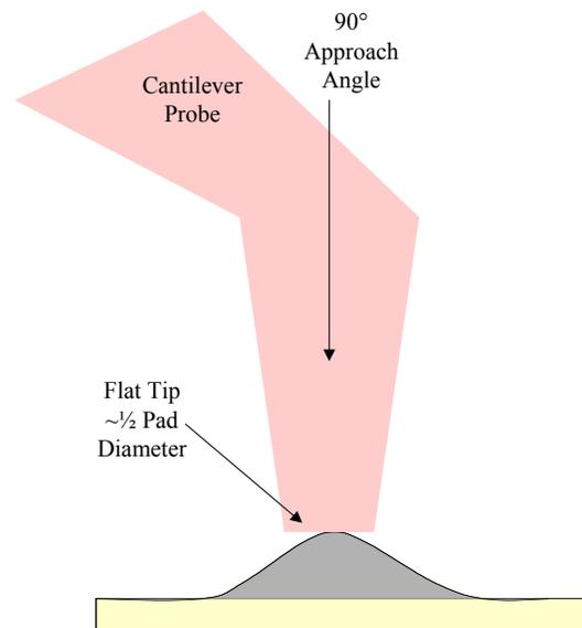
While cantilever beam probes can provide an effective probing solution for perimeter arrays, high-density area bump arrays are more suitable to be probed by one of the wide range of vertical probing technologies available.
