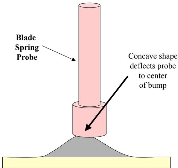
One approach to probing bumped wafers is to use blade spring probes or pogo pins with concave probe heads. This technology ensures that the probe body automatically centers on the bump when overdrive is applied to the probe system. While quite effective, these probes are relatively large (21 mils diameter) and hence can only be used in lower density/pitch applications.
