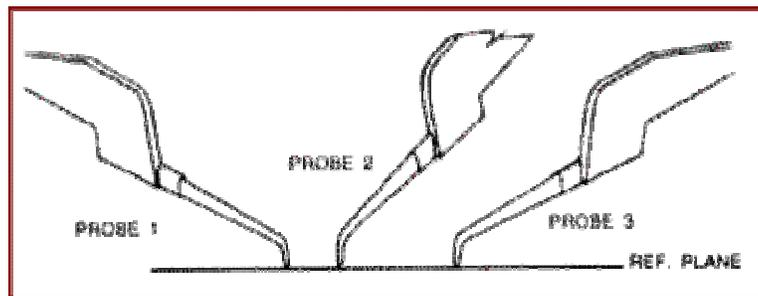
Figure 3 shows all three probes on the same reference plane and at the proper planarization depth.
