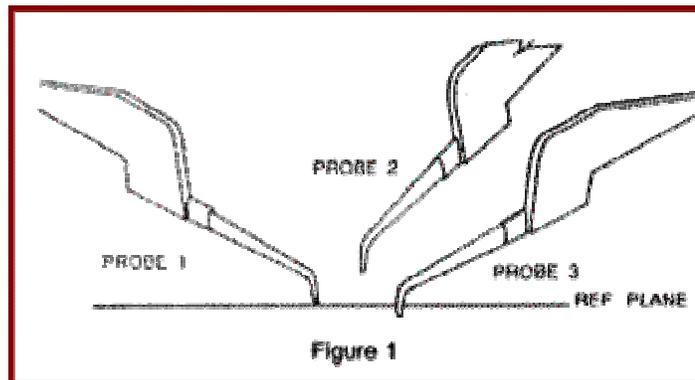
Figure 1 shows three probes; each of which having its probe point at different positions relative to each other. Only one probe (probe 1) is at the correct depth on the reference plane (planarization depth "D") while the other probes are either low or high.
