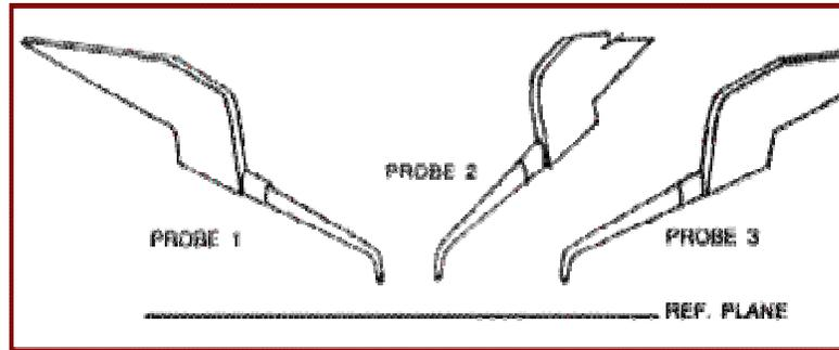
Figure 2 shows all three probe points to be on the same plane relative to each other but are not at the correct planarization depth.
