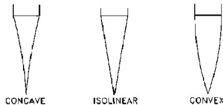
*Figure 19. Probe tip etch.*
