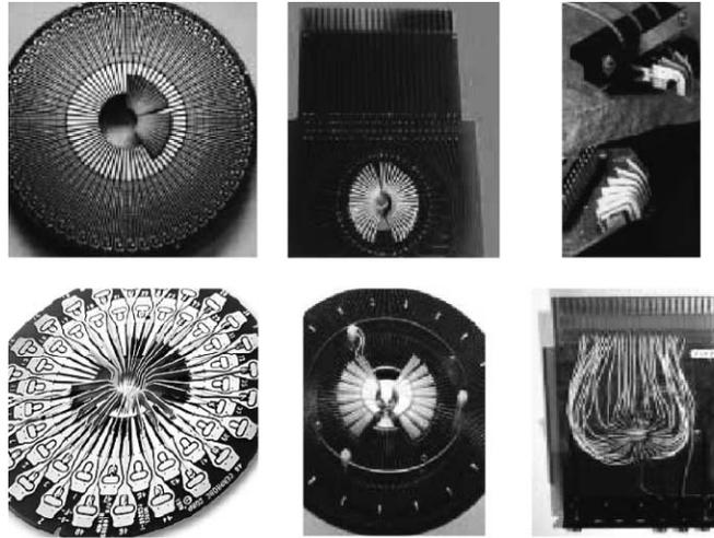
*Figure 5. Different types of ceramic blade probe cards.*
