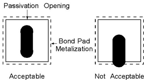
**Figure 22. Proper scrub alignment.**
