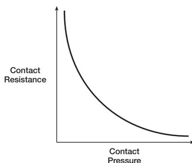
**Figure 20. Relationship between contact force and C<sub>Res</sub>.**
