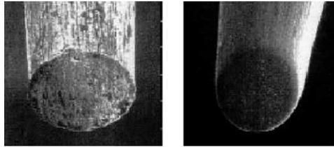
*Figure 18. Flat and semi-radius tip shapes.*
