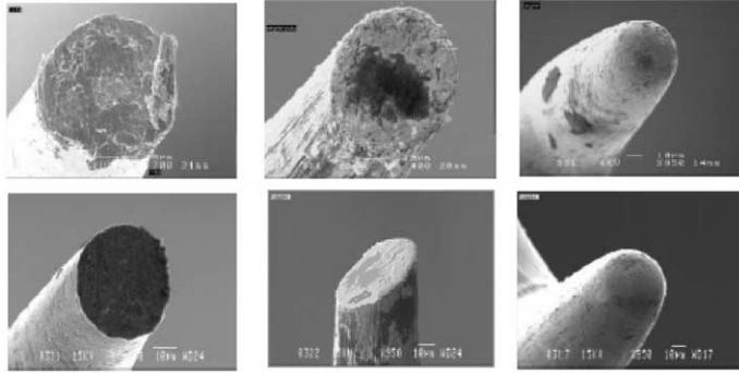
**Figure 28. Before and after a non-abrasive clean.**
