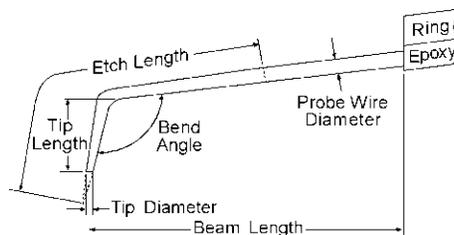
*Figure 17. Probe geometry diagram.*
