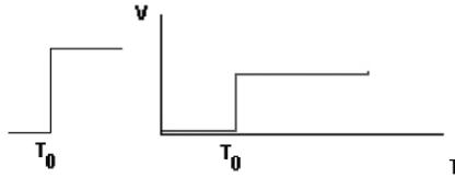
***Resistor response to a step function.***
