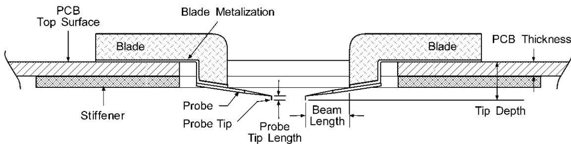
**Figure 3.** Blade probe card with blades attached.
